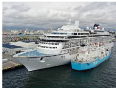
Photos: Shore Power supply (Left) and LNG bunkering at FUKUOKA © KEYS Bunkering West Japan KK
